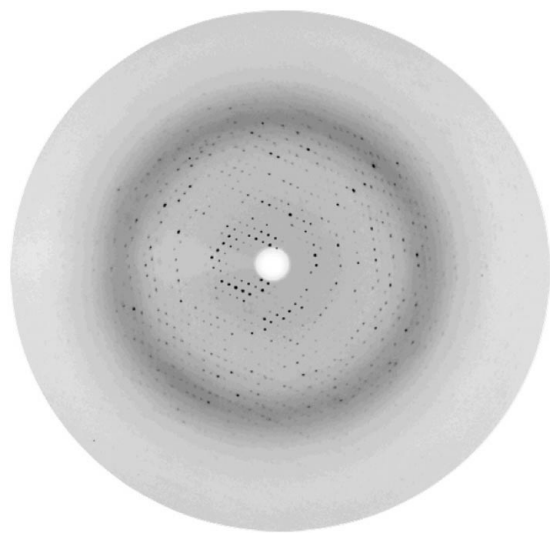
Figure 3 The diffraction pattern of AK III. Data were collected at APS BioCARS beamline 14-D at a detector distance of 175 mm and a 15 s exposure. The resolution at the edge of the figure is approximately 2.0 Å.
